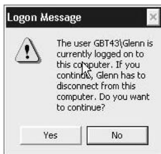
FIGURE 6-3: Windows Terminal Services needs to take over the remote computer's Windows login session
