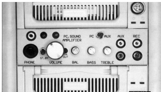
Separate PCB (terminal PCB) in a metal case, that is attached to their PC's back panel.
